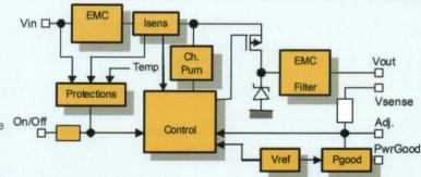
Input and output EMC filters are integrated to simplify module implementation directly on the digital board with only one additional component (resistor for output voltage adjustment).
