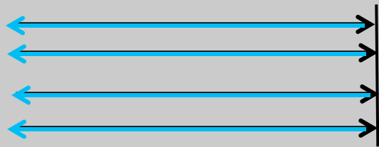
Deformable mirror Focal length: infinity
