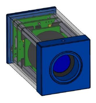
Ultra compact Intensified Camera, NIT Native Wide Dynamic Range Sensor inside, Intensifier tube (Gen 2), USB 3.0 output, CS/C mount Interface
