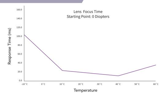
You can see at 10°C, it takes about 20ms or less to snap into any focal point. For reference, a high end DSLR camera with AF would take 300+ ms to do the same.
